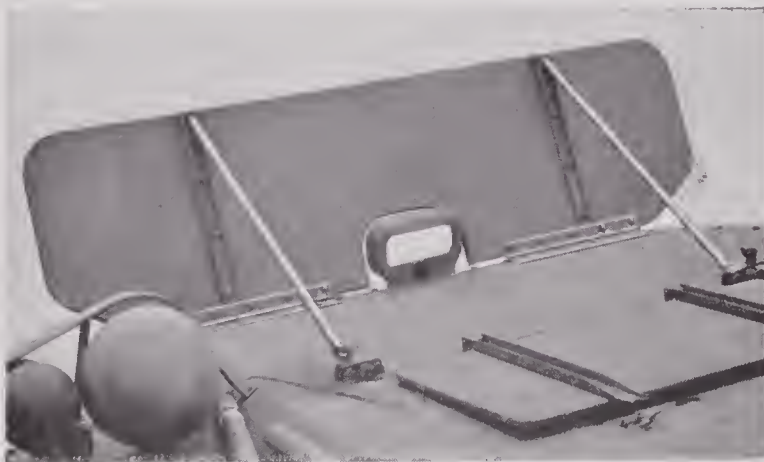
FIGURE 35. First surf plate made of unreinforced plywood and secured with piano hinges.
